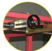
张力调整装置 Tension adjustment device
